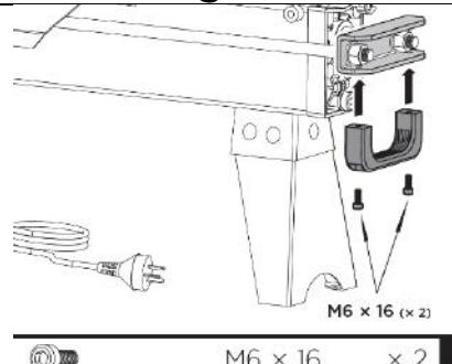
**A. Mounting the lifting handle:** Attach the lifting handle to the U-bracket with two M6x16 screws.
