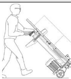
To move the log splitter over short distances, hold it by the transport handle and tilt it slightly - see illustration on the left.
