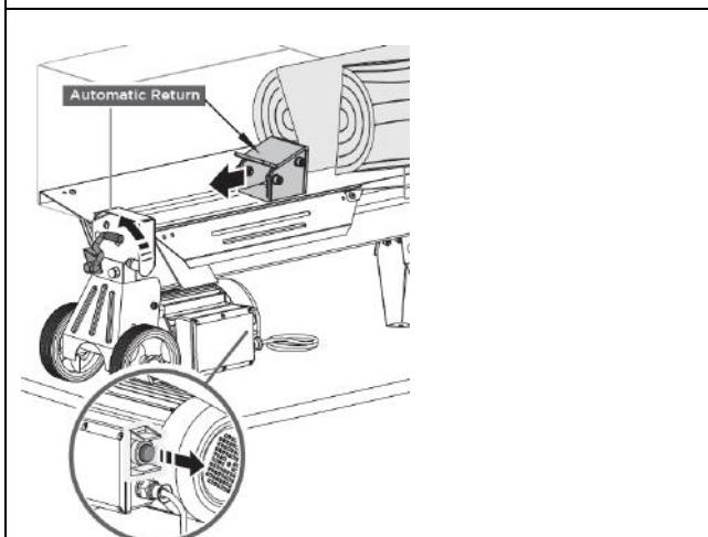
The trigger-controlled locking device is designed to prevent accidental lowering of the hydraulic control lever.
