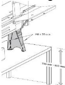
Before putting the wood splitter into operation place it on a 72–85 cm high, stable and level workbench and fasten the support leg with two screws (M8x35) as shown in the picture on the left.
