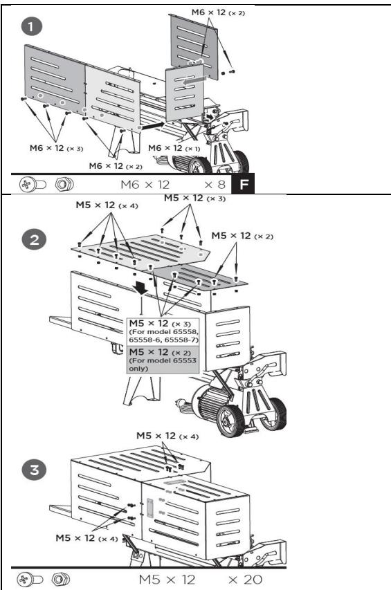
**A. Attaching front guard plates, left guard plate and rear guard plates:** Fix the front guard plate, the left guard plate and two rear guard plates with screws M6×12 and nuts to the log tray and the bottom plate (1).
