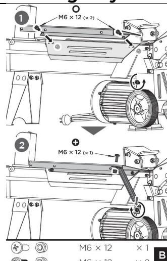
**A. Fastening the guard bottom plate:** Mount the guard bottom plate to the rear guide plate and secure it with the two socket head cap screws M6×12 and the lock nuts. Loosen the socket head cap screw and the large washer on the wheel bracket, insert the open end of the support strut 2 between the large washer and the wheel bracket and tighten the screw. Connect the upper end of support strut 2 to the guard bottom plate with a cross recessed pan head screw M6×12 and lock nut M6 and tighten.
