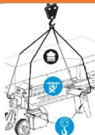
When using a crane for lifting (e.g. when loading the splitter onto a truck), attach the hoist only to the intended places - see illustration on the left.
