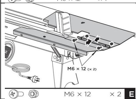
**D. Connecting log tray right and left:** Connect log tray 1 and 2 with two screws M6×12 and lock nuts.
