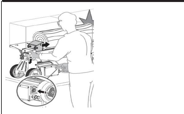
The log splitter is equipped with a two-hand control. The left hand controls the hydraulic control lever, the right hand the pressure switch (see illustration on the left). If one hand is missing, the log splitter "freezes".
