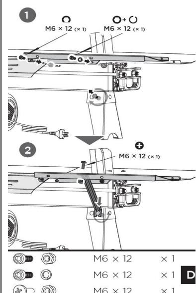
**C. Log tray left:** Align the two mounting holes of log tray left with the holes on the front of the splitter. Insert a socket head cap screw M6×12 and a spring washer 6 into the mounting hole on the right side, another socket head cap screw M6×12 and lock nut M6 on the left side and tighten both screws firmly.
