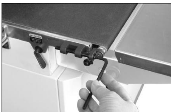
Figure 8-3: belt tension adjustment
