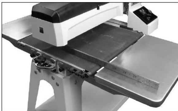
Figure 6-4: extension table alignment
