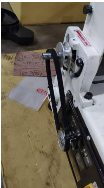
1.Put the belt on the drive wheel.
