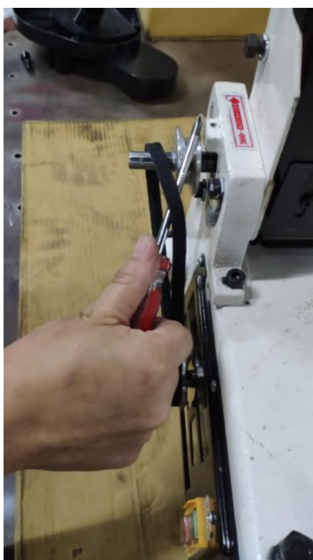
2.Use a screwdriver through the belt.
